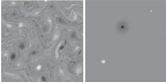
FIG. 1. Vorticity field at  $t = 4$  (left) and  $t = 160$  (right) in one representative simulation. A linear gray scale is used, with the highest positive vorticity being white. Only  $1/16$  of the domain is shown.
