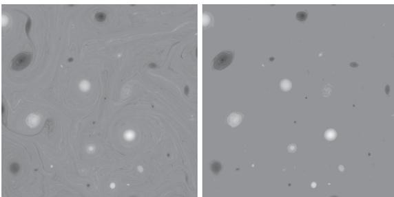
FIG. 2. Full vorticity field  $\omega(\mathbf{x}, t = 16)$  (left) and its corresponding coherent part (right). Only  $1/16$  of the domain is shown.
